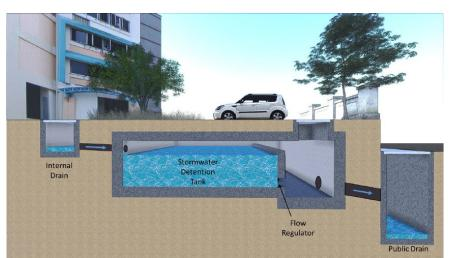
Example of simple stormwater detention system.
