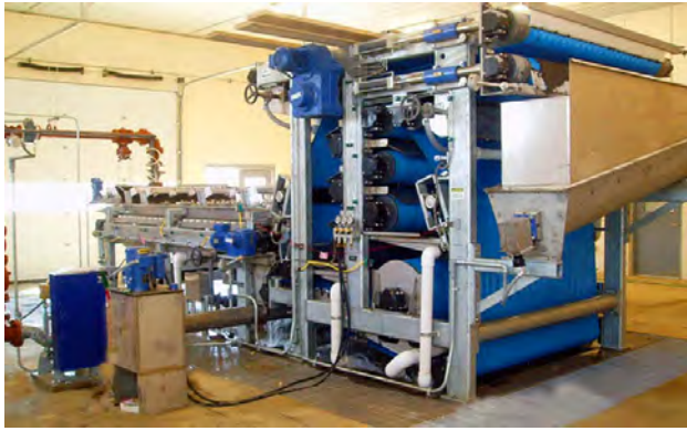
(a) Belt Filter Press (courtesy of BDP Industries)
