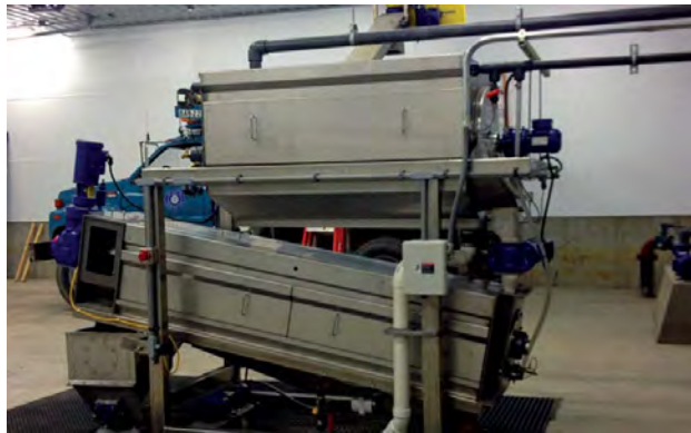
(c) Screw Press (courtesy of BDP Industries)
